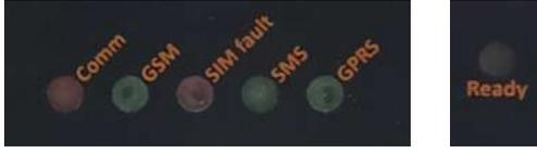
LEDs placed on the front panel of the Modem displays communication status.
