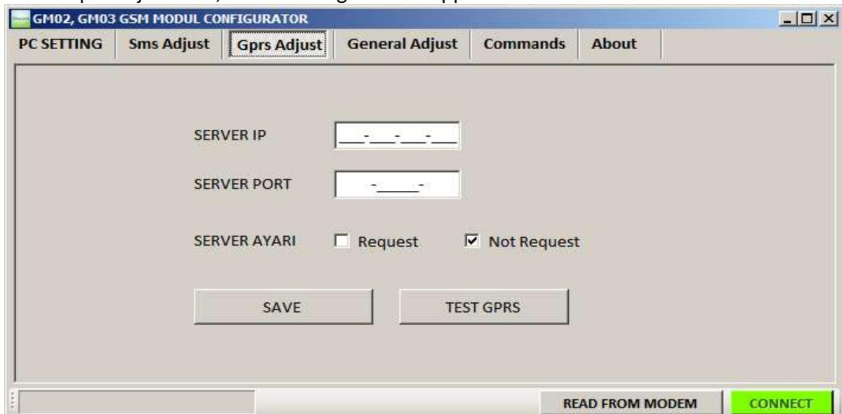
You can set the IP and PORT numbers of the server for GPRS reporting. When entering the IP and PORT numbers, the gap should be written to 0.
