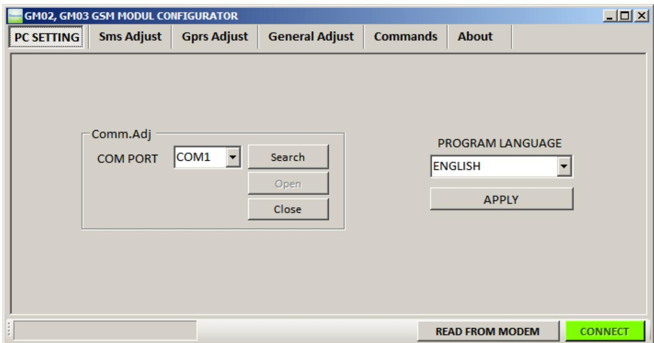
This connection remains active as long as data communication.. If there is no communication between PC program and GSM modem during 20 seconds, the connection will be lost. You should click "CONNECT" button to link back.
